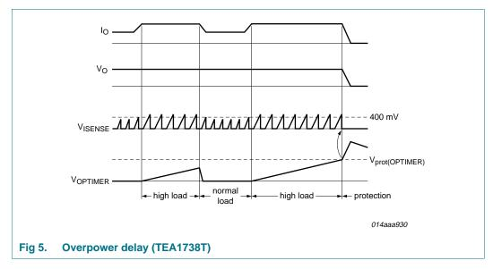
In the TEA1738T when the  $V_{prot(OPTIMER)}$  voltage is reached the device is restarted. The TEA1738LT is latched in an off state when the  $V_{prot(OPTIMER)}$  voltage is reached.
