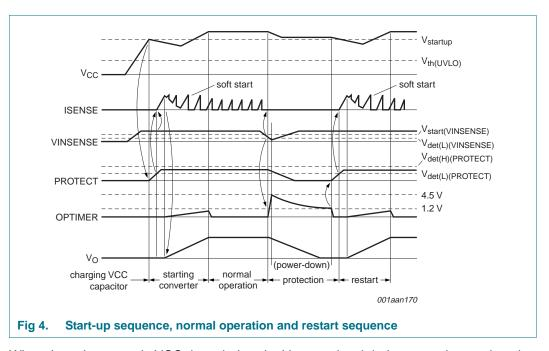
When the voltage on pin VCC drops below the  $V_{th(UVLO)}$  level during normal operation, the controller stops switching and the TEA1738T enters Restart mode. In Restart mode the driver output is disabled and the VCC pin voltage is recharged via resistor R3 to the rectified mains voltage. For the TEA1738LT a VCC undervoltage, which does not occur during a start-up event, latches the IC in an off-state.
