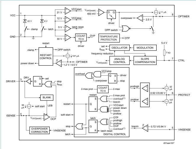
(1) In the TEA1738LT the overload signal switches the IC to the latched-off state. In the TEA1738T the overload signal triggers the restart timer.
